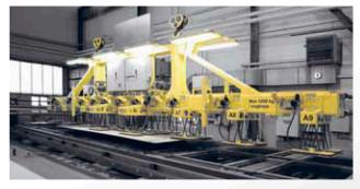
Skanveir's magnetic and vacuum lifters can be attached to cranes, forklifts or transfer systems. Our reliable equipment requires minimum maintenance.
