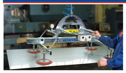
The Dumbo vacuum lifter is a light, easy-to-use, and handy tool for handling metal sheets.
